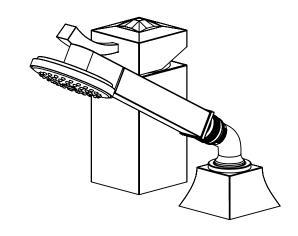
**ICE** Pressure Balance Deck Mount Mixing Valve with Hand Held Shower & Build-in Vacuum Breaker Model: 5RRBICL-XX-XX
