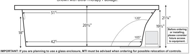
INSTALLATION: Add 1"-3" to height of tub for bedding compound. MTI recommends Quickrete Sand Mix. Air Baths add approximately 2"-3" to height of tub. Please measure tub before building tub decking. Suction and control locations may vary. Drawing shows best pump location. Alternate locations available — call MTI for details. Measurements are ± 1/2" and are subject to change without notice. Data herein supersedes
