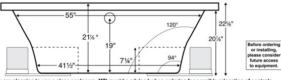
IMPORTANT: If you are planning to use a glass enclosure, MTI must be advised when ordering for possible relocation of controls.
