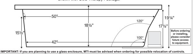
INSTALLATION: Add 1"-3" to height of tub for bedding compound. MTI recommends Quickrete Sand Mix. Air Baths add approximately 2"-3" to height of tub. Please measure tub before building tub decking. Suction and control locations may vary. Drawing shows best pump location.
