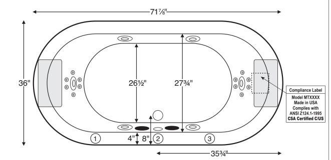
Numbered locations on tub deck are possible Fill-Flush, Hand-Held Shower or Breda locations. If location 2 is chosen for Fill-Flush, the detergent feeder will need to be offset to the left or the right.
