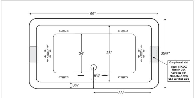
NOTE: Top deck/rim of tub is curved and not designed to mount faucetry.
