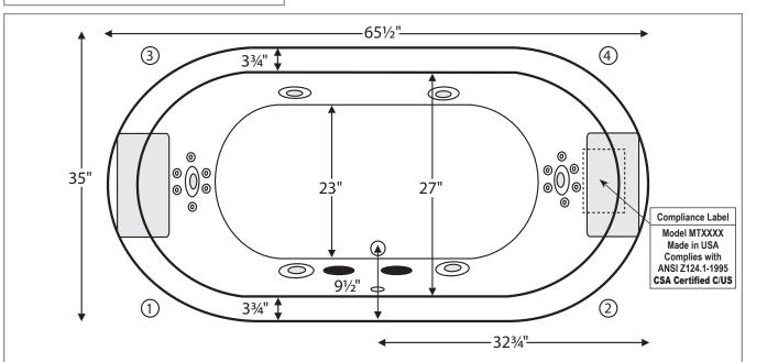
Numbered locations are possible stub out locations for Fill-Flush, Hand-Held Showers or Breda valves.
