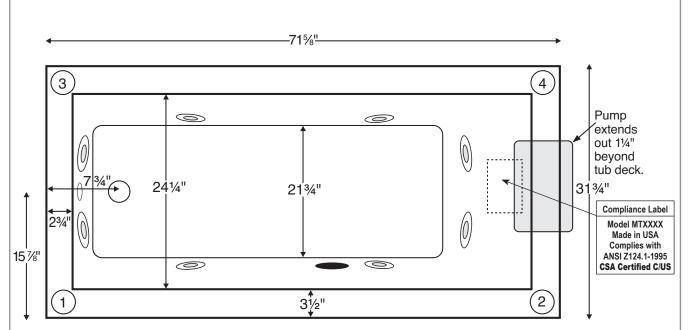
Numbered locations on tub deck are possible Fill-Flush, Hand-Held Shower or Breda locations. Pump extends out approximately 11/4" beyond tub deck.
