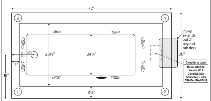
Numbered locations on tub deck are possible Fill-Flush, Hand-Held Shower or Breda locations. Pump extends out approximately 2" beyond tub deck.
