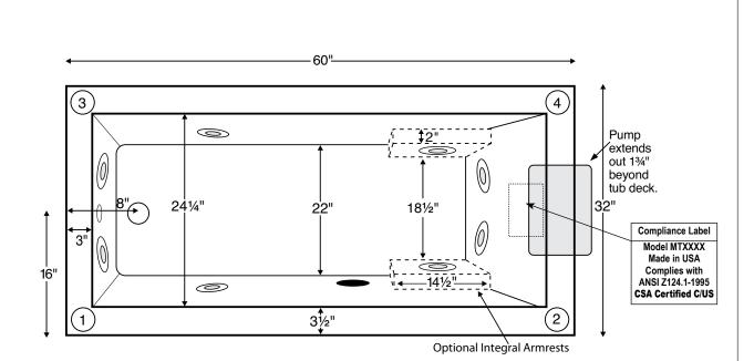
Numbered locations on tub deck are possible Fill-Flush, Hand-Held Shower or Breda locations. Pump extends out approximately 1 3/4" beyond tub deck.
