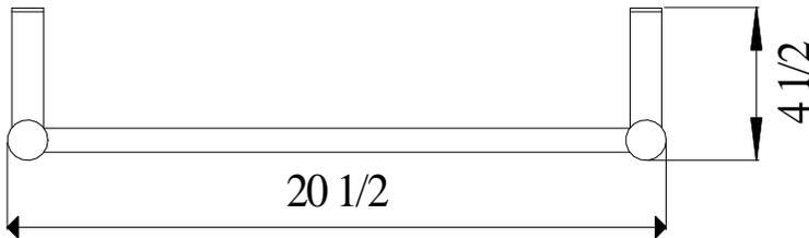
For construction with wall studs on 16 in. centers, the header is located between the studs for the right side mounting. For construction with wall studs on centers greater than 19-1/2 in. provide secure header as shown.
