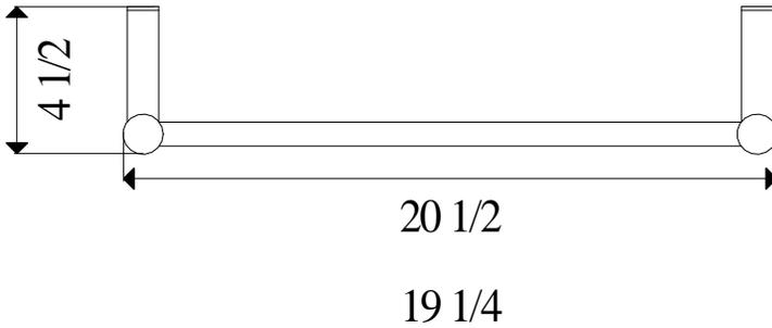
For construction with wall studs on 16 in. centers, the header is located between the studs for the right side mounting. For construction with wall studs on centers greater than 19-1/2 in. provide secure header as shown.
