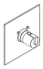
R10 3/4" or 1/2" Thermostatic Mixing Valve Model: 4D/4MRT0 XX-XX
