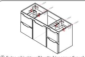
③ Fasten cabinet to wall by attaching screws through the bracket holes, and by attaching the lower brackets. Use a spirit level to ensure vanity is leveled.
