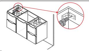
① Drill through the hole in the corner bracket on the backboard or as shown. Mark the wall according to the holes at your preferred height and drill holes in the wall.
