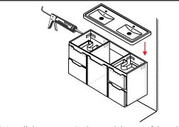
(5) Install the counter. Seal around the top of the cabinet with clear silicone sealant. Do not over apply. Allow to dry for over 24 hours for proper curing.
